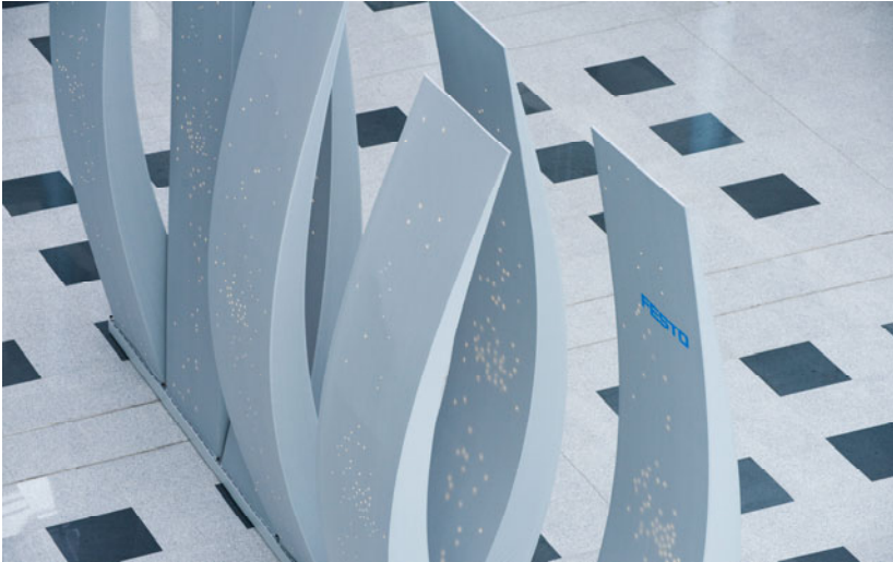
Fig. 4. Top: The InteractiveWall at the Hannover Messe 2009 displaying real time behavior by swinging its body back and forth, displaying patterns of light on its skin, and projecting localized sound.
