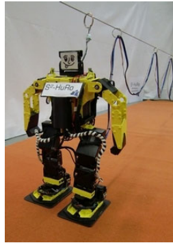
Fig. 8. One of the four test setups - S2-HuRo self-stabilization experiment on orange soft carpet
