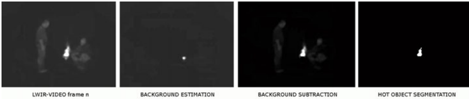
Fig. 2. Hot object segmentation by background subtraction and histogram-based dynamic thresholding
