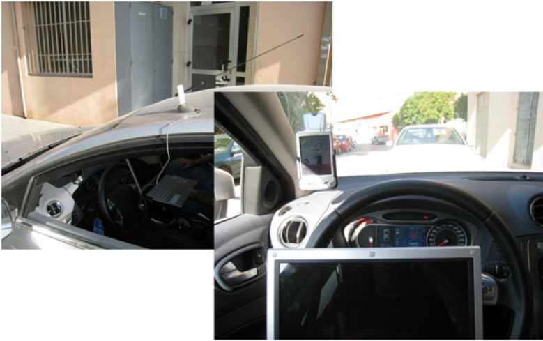
Fig. 2. Images of the experiment to determine the radio signal attenuation due to distance between vehicles
