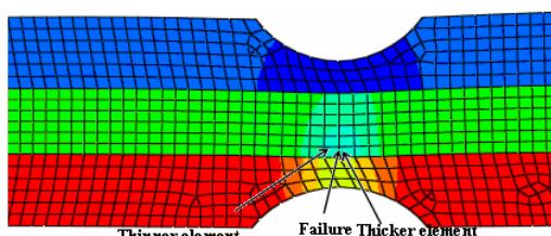
**Fig. 3.** Failure location in TWB with longitudinal weld
