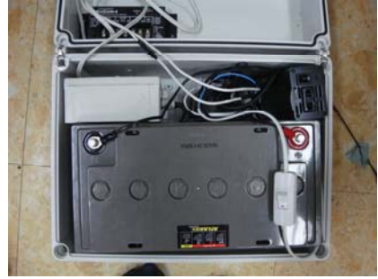
Fig. 9. Soil sensor receiver, solar battery
