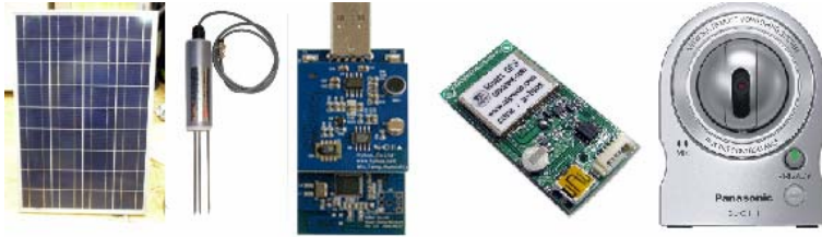
Fig. 7. Solar cell, soil sensor, network sensor node, GPS module and CCTV camera in the FMSS
