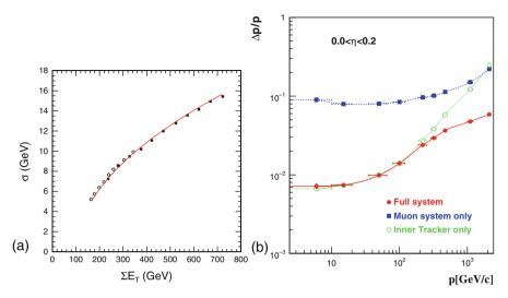
Fig. 5.16 (a) Missing transverse energy resolution as a function of the sum of the transverse energy,  $\sum E_T$ , for minimum-bias and soft QCD events at low luminosity [23]. (b) Resolution for muons in the central detector, reconstructed with the muon system only, the tracker only and the combined measurement [23]
