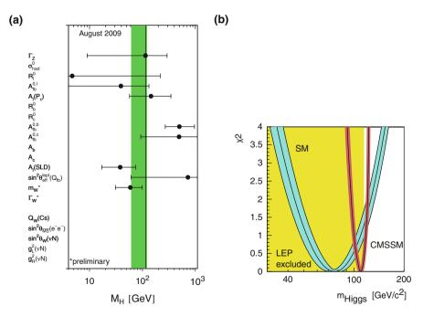
**Fig. 4.11** (a) Electroweak measurements and their individual constraints on the Higgs mass [12]. (b) The sensitivity of the SM and CMSSM Higgs boson *h* expressed in terms of  $\Delta \chi^2$  of the combined fi to the electroweak data [48]
