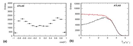
**Fig. 6.8** (a) Distribution of  $\cos \theta^*$  for reconstructed electron pair events in the Z pole region [2]. The monte carlo events are generated with the PYTHIA [37] program and passed through the ATLAS detector simulation. (b) Simulated rapidity distribution of  $e^+e^-$  pairs [2]. The upper line shows the distribution for all events, the lower line only events with correctly reconstructed quark direction
