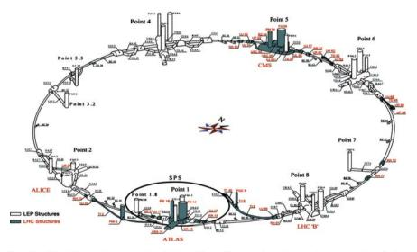
**Fig. 5.1** The LHC underground installation. The ATLAS and CMS experiments are installed at opposite sites of the main ring at access points 1 and 5. ALICE and LHCb are close to the ATLAS site at point 2 and 8, respectively. The protons are injected from the SPS into the LHC via beam transfer lines. Eventually, the protons are stopped at the end of the beam lifetime into a beam dump system at point 6
