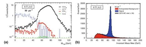
Fig. 6.1 (a) Simulated transverse mass distribution in the  $W \rightarrow ev_e$  channel for an integrated luminosity of  $50 \text{ pb}^{-1}$  [2]. (b) Invariant di-electron mass measured in  $Z \rightarrow e^+e^-$  events and the corresponding background, again for  $50 \text{ pb}^{-1}$  [2]
