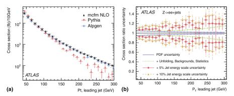
Fig. 6.2 (a) Parton level comparison of the  $p_T$  of the leading jet in  $Z \to \mu^+ \mu^- + jets$  Monte Carlo samples for LO and NLO predictions [2]. (b) Systematic uncertainty on hadron level  $p_T$  of the leading jet in  $Z \to e^+e^- + jets$  events for  $\mathcal{L} = 1 \text{ fb}^{-1}$  [2]. If the dominant jet energy scale uncertainty can be reduced below 10%, sensitivity to NLO predictions is possible
