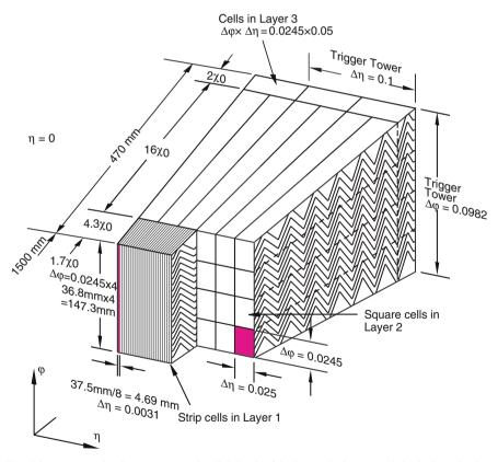
**Fig. 5.9** Segmentation in  $\Delta \eta \times \Delta \phi$  and radial depth of the LAr calorimeter cells in the barrel. Also indicated is the size of the calorimeter trigger towers which combine larger angular areas [1]
