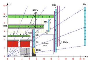
Fig. 5.12 Schematic view in the r - z plane of one quarter of the ATLAS muon detectors [1], with MDT chambers in barrel and endcap inner, middle and outer layer (BIL, BML, BOL, EIL, EML, EOL), the CSC and TGC detectors in the endcap region, as well as the RPC trigger layers attached to the barrel middle and outer MDTs
