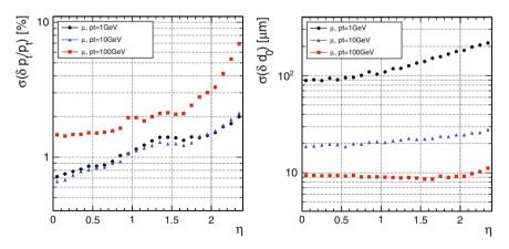
Fig. 5.14 Expected momentum and transverse impact parameter resolution of single muon tracks of three different energies, simulated for the CMS tracking system in different  $\eta$  regions [23]
