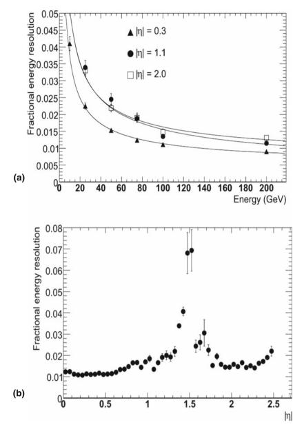
Fig. 5.10 (a) Expected energy resolution for electrons in different  $\eta$  ranges as a function of energy [1]. (b) Relative energy resolution for 100 GeV electrons as a function of  $\eta$ . The resolution is rather uniform except in the transition region between barrel and endcap [1]
