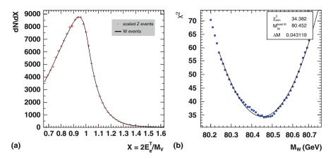
Fig. 6.3 (a) Comparison of the rescaled  $E_T$  spectrum of electrons in  $Z \to e^+e^-$  events 1 fb<sup>-1</sup> [9]. (b) The corresponding  $\chi^2$  distribution of the W mass derived from this spectrum
