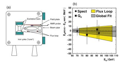
**Fig. 2.2** (a) Schematic view of the LEP reference dipole magnet with NMR probe and flu loop installed. (b) Comparison of the beam energy measurements using the LEP spectrometer, the flu loop and the tune shift,  $Q_s$ , with the measurement by the NMR probes. Also shown is the result of the global calibration fi [4]
