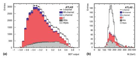
**Fig. 6.5** (a) Boosted decision tree (BDT) output for single-top signal and background [2]. (b) Leptonic top quark mass distribution applying cut on the BDT output at 0.6 [2]
