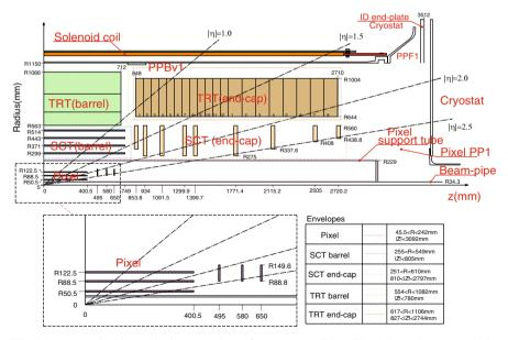
Fig. 5.6 Geometrical layout in the r - z plane of one quarter of the ATLAS inner detector with the pixel, SCT and TRT sub-detectors [1]
