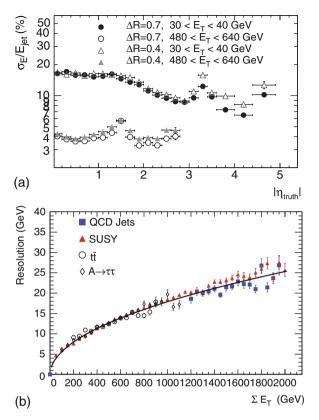
**Fig. 5.11** (a) Expected jet energy resolution for seeded iterative cone jets with different cone size and energy range [1]. (b) Resolution of the reconstructed transverse missing energy as a function of the sum of the transverse energy in the event [1]. Different event samples are used to evaluate the resolution at various transverse energy scales
