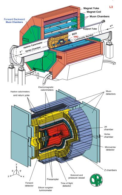
Fig. 2.4 Schematic view of the L3 and OPAL detectors
