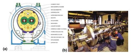
**Fig. 5.3** (a) Cross-section through a LHC dipole magnet inside its vacuum vessel with the two beam pipes, the cold screen and the superconducting coils [3]. (b) One of the four superconducting cavities that are combined in each of the two RF modules which supply the 400 MHz RF power to the proton beam
