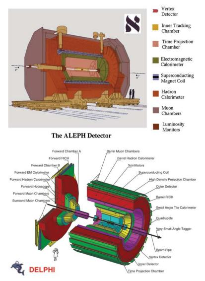
Fig. 2.3 The ALEPH and DELPHI detectors at the LEP collider
