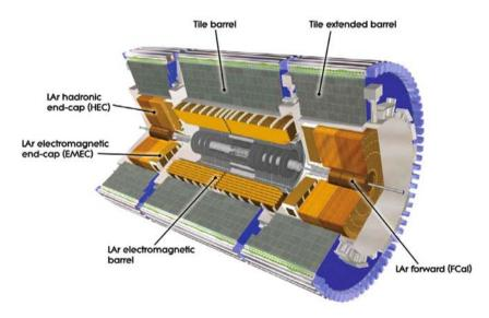
**Fig. 5.8** The ATLAS Liquid Argon calorimeters consist of the electromagnetic barrel and endcap calorimeters, a hadronic endcap and a forward calorimeter. They are installed in metal cryostats onto which the front-end electronics is mounted. The ATLAS calorimetry is completed by a hadronic Tile calorimeter in the barrel and forward region
