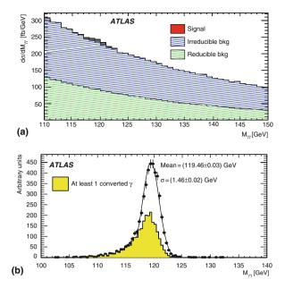
Fig. 7.2 (a) Di-photon invariant mass spectrum after the application of cuts of the inclusive analysis, without additional requirements on jets,  $E_T^{\text{miss}}$  or leptons [5]. (b) Invariant mass distribution for photon pairs from  $H \rightarrow \gamma \gamma$  decays with  $M_{\text{H}} = 120$  GeV after trigger and identificatio cuts [5]. Events with at least one converted photon are displayed as the shaded histogram
