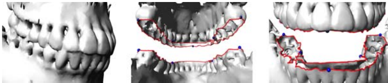
Fig. 4. Results of interactive segmentation path planning (model #1). Selected control points are shown as blue points and the searched segmentation paths are red curves.
