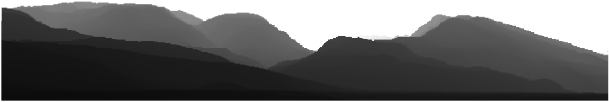
Fig. 1. 70° wide by 40° tall section of unwrapped synthetic panorama, with intensity proportional to distance
