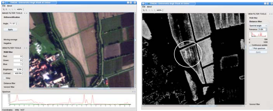
Fig. 5. Left. Orthorectified frame in the visible band from a different area of Aquileia. Right. The same area. Spectral angle distance filtering of frames taken in the near infrared. The reference spectral data (panel on the right) are from a known building. A buried structure is apparent (circled), not distinguishable in the visible band.
