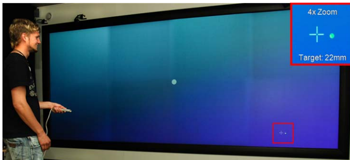
Fig. 2. Comparing absolute input and Adaptive Pointing at a large, high-resolution display. Device: infrared laser-pointer, distance: 3 meters.
