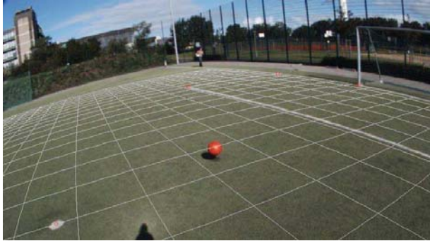
Fig. 2. Grid overlay of a homography between the image plane and the field plane. Observe the fine correspondence near the line in front of the goal.
