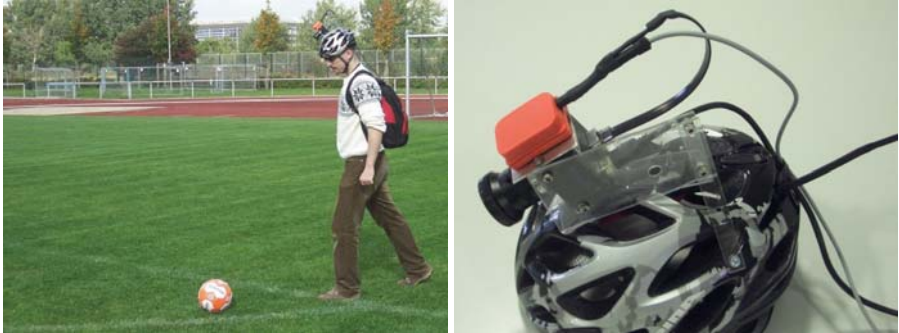
Fig. 1. The proposed sensor setup with a wide angle camera and an inertial sensor
