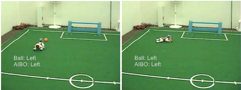
Fig. 5. The images show the behavior of the AIBO robot during ‘GO&SHOOT’ testing task. The left image shows part of the ‘GO’ task while the right image shows part of the ‘SHOOT’ task. The task was tested with ball and robot at different initial positions.
