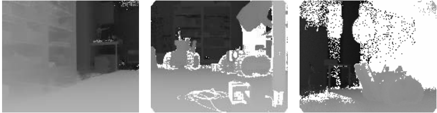
(d) Unfiltered distance image with objects removed, for comparison (e) Proposed method: dark pixels removed – 13.1 % d. p. (f) Proposed method: very little noise remains – 44.9 % d. p.
