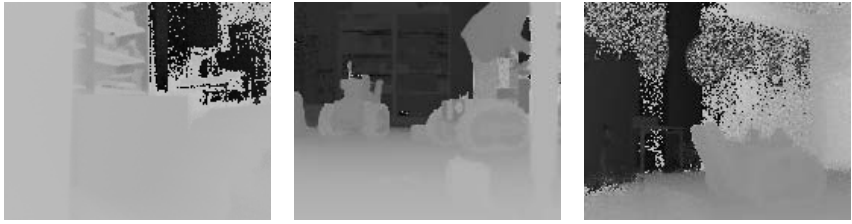
(a) Unfiltered distance image: Dark obstacles in the back appear too close (b) No wrap-around, but noisy and too close (c) Sun causes error and random noise due to dark material
