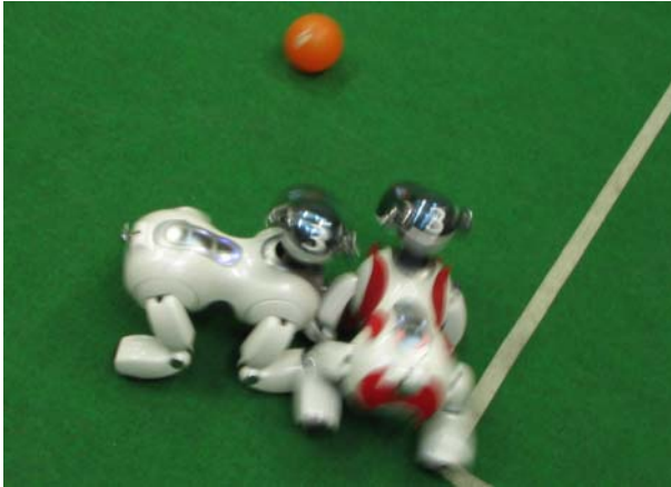
Fig. 1. One robot colliding with another, which is a very common situation in a robot soccer game. Both are unable to proceed in the desired direction; hence, the result is failure in the task.
