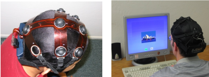
Fig. 1. 6 Channel B-Alert® ( right ) system wirelessly records EEG and EKG. AMP set-up ( left ) measures performance and physiology during a battery of neurocognitive tests.
