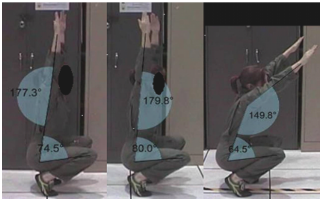
Fig. 2. Example: Posture while crouching and reaching overhead in oversized (Left), appropriately Sized (Center) and undersized (Right) Flight Suits
