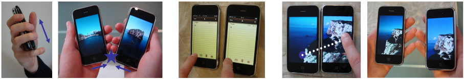
Fig. 1. a) Shaking b) Bumping c) Simultaneous Button Pressing d) Stitching e) Touching
