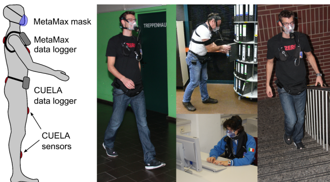
Fig. 1. Measurement instrumentation during activity protocol
