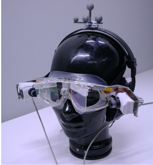
Fig. 1. Head-mounted eyetracking system [13] and headphones for the virtual acoustics
