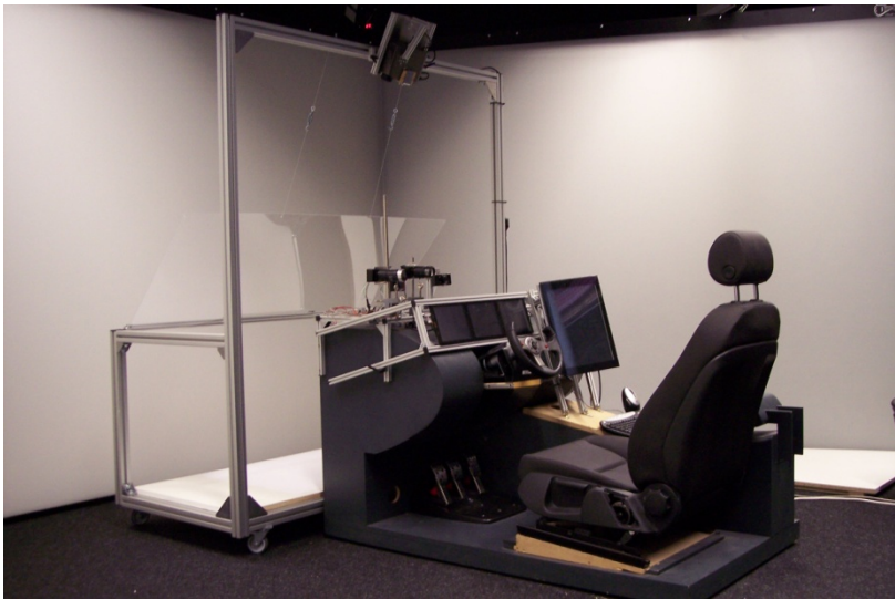
Fig. 3. System overview: mock-up and mounted displaying areas
