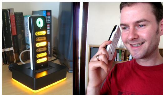
Fig. 4. The final design showing the black internet ‘face’ when docked and the white landline ‘face’ in use
