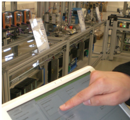
Fig. 7. SmartFactory KL – the comprehensive user interface running on the PaceBlade touch screen (foreground) is used to steer devices of the production environment (background)
