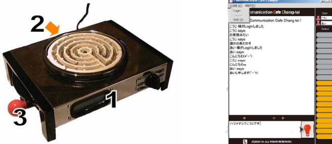
Fig. 4. The communication grill (all in one edition): an LCD (1) to indicate an IP address, an Ethernet port (2) to receive operating signals from chat applications, and an indicator lamp (3) (Left). The Communication Grill Application: a screen shot of the chat application. The bar meter indicates the remaining time before power shutdown, implemented on the right side of the window (Right).
