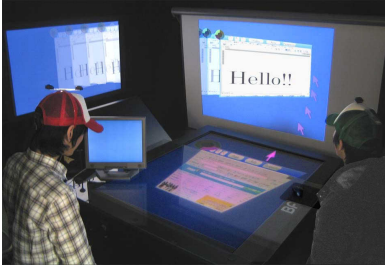
Fig. 6. Cursor-motion and window jumping caused by gaze input
