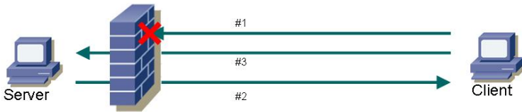
Fig. 3. UDP hole punching with netcat
