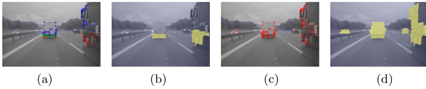
Fig. 6. Detection and segmentation results of preceding and oncoming objects. Monocular vision (a,b) is only able to detect the lower parts of the preceding objects; the oncoming object is not detected at all. Stereoscopic vision (c,d) does not suffer from these limitations. (Color encoding as in Figure 5.)
