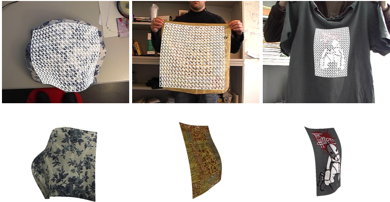
Fig. 1. 3D Reconstruction of non-rigid objects from an individual image and a reference configuration. Results were obtained in closed-form, without any initial estimate. Top: Recovered mesh overlaid on the original image. Bottom: Re-textured side view of the retrieved surface.
