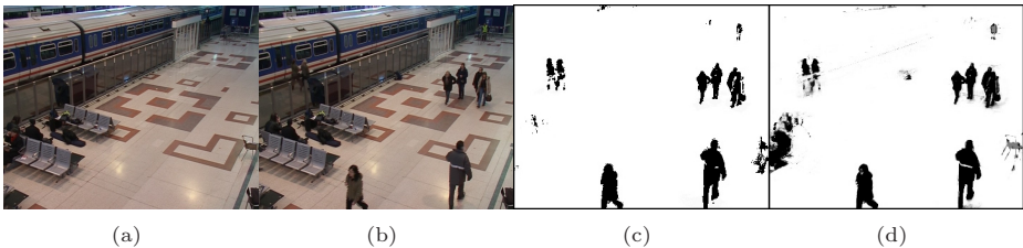
Fig. 6. PETS 2006 Dataset. (a) Initial frame of the video, used as background model. (b) Frame number 2800. (c) The background subtraction of [1]: The abandoned bag in the middle of the scene has mistakenly been integrated into the background. (d) Our method correctly segment the bag, the person who left after sitting on the bottom left corner, and the chair that has been removed on the right.
