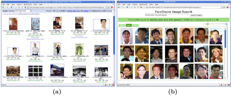
Fig. 1. Results for the query “smiling asian men with glasses,” using (a) the Google image search engine and (b) our face search engine. Our system currently has over 3.1 million faces, automatically detected and extracted from images downloaded from the internet, using a commercial face detector [1]. Rather than use text annotations to find images, our system has automatically labeled a large number of different facial attributes on each face (off-line), and searches are performed using only these labels. Thus, search results are returned almost instantaneously. The results also contain links pointing back to the original source image and associated webpage.
