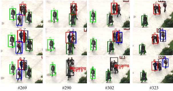
Fig. 7. Disposal of interactions or “merge/split” among targets: The first row is the tracking results of multiple independent color-based trackers [29]. The second row is the results of multiple independent Ensemble Trackers [1] and the the third is our tracking results.
