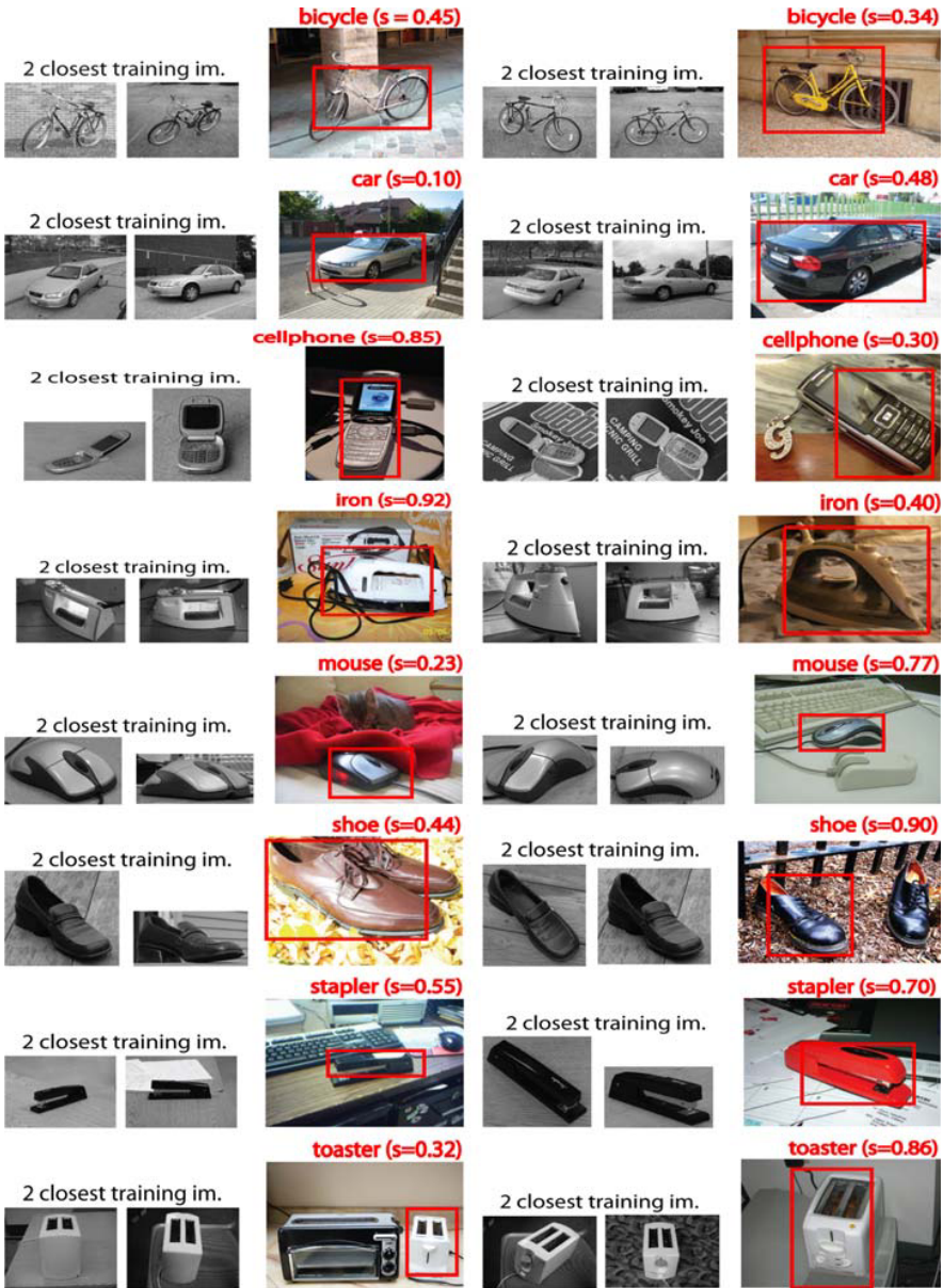
Fig. 9. Estimated pose for each object that was correctly classified by our algorithm. Each row shows two test examples (the colored images in column 3 and column 6) from the same object category. For each test image, we report the estimated location of the object (red bounding box) and the estimated view-synthesis parameter s . s gives an estimate of the pose as it describes the interpolating factor between the two closest model (canonical) views selected by our recognition algorithm. For visualization purposes we illustrate these model views by showing the corresponding training images (columns 1-2 and 4-5). (This figure is best viewed in color with PDF magnification.)
