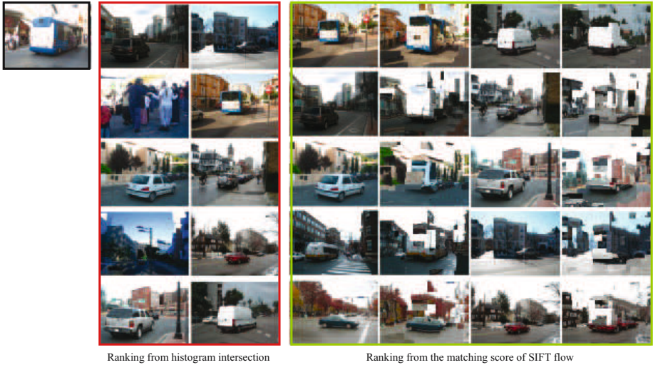
Fig. 7. Alignment typically improves ranking of the nearest neighbors. Images enclosed by the red rectangle are the top 10 nearest neighbors found by histogram intersection, displayed in a scan-line order (left to right, top to bottom). Images enclosed by the green rectangle are the top 10 nearest neighbors ranked by the minimum energy obtained by the alignment algorithm. The warped nearest neighbor image is displayed to the right of the original image. Note how the returned images are re-ranked according to the size of the depicted vehicle by matching the size of the bus in the query.
