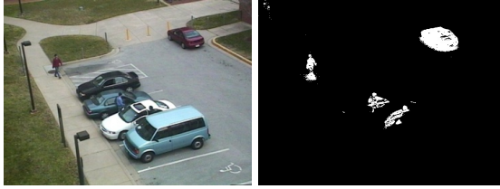
Fig. 2. A frame from a parking lot sequence and its corresponding foreground regions detected using background subtraction. Here, parked cars introduce significant occlusion and door openings lead to many false alarms.
