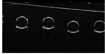
Fig. 6. B-scan showing the cross-sections of nylon wires in the aqueous environment at \alpha = 10^\circ . The white line in the upper part corresponds to the sealing glass plate.
