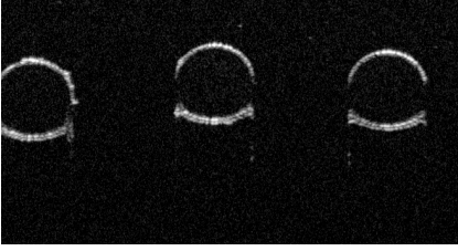
Fig. 7. B-scan showing the cross-sections of nylon wires in the aqueous environment at \alpha = 0^\circ
