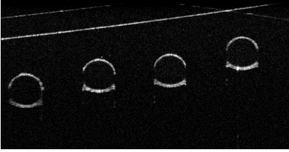
Fig. 5. B-scan showing the cross-sections of nylon wires in the aqueous environment at \alpha = -10^\circ . The white line in the upper part corresponds to the sealing glass plate.
