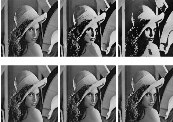
Fig. 2. The rows present the images processed by the defined operator at scales 1 and 0.1, respectively. The columns represent 1, 10 and 50 iterations.
