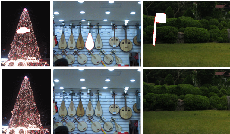
Fig. 4. The results of band matching: Upper line is input images and lower line is results of band matching. Computation time was 15, 26, 200 seconds, respectively. The number of band pixels is 1396, 1576, 2324 pixels, respectively. When [4] was applied, it took 420, 780, 1800 seconds.
