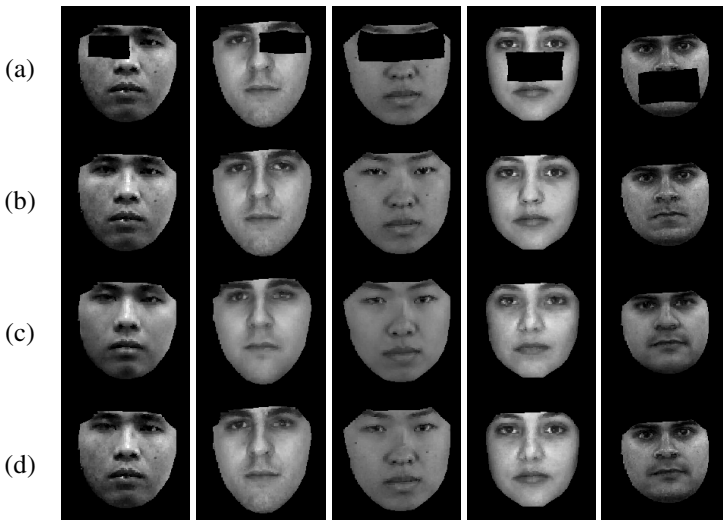
Fig. 4. Reconstruction results obtained using DCM method: (a) occluded facial images, (b) original facial images, (c) reconstructed facial images using global texture DCM only, and (d) final reconstruction results using both global texture DCM and local texture DCM
