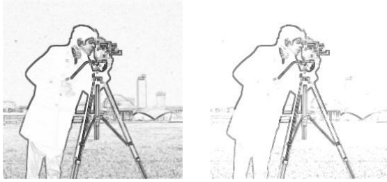
Fig. 3. Fuzzy morphological edge images for (\mathcal{C}, \mathcal{I}) = (T_M, I_{KD}) (left) and (\mathcal{C}, \mathcal{I}) = (T_W, I_W) (right)
