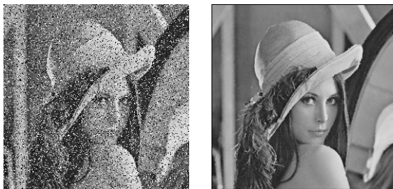
Fig. 5. The Lena image with 20% impulse noise (MSE = 3309,40), and the result of the FIDRM filter (MSE = 30,57)
