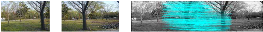
Fig. 2. Original images (the left two images) and SIFT feature matches extracted from a pair of images (right)
