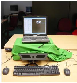
Fig. 3. Set-up for the usability study (including a third mouse for the leader of the experiment to start and stop applications)
