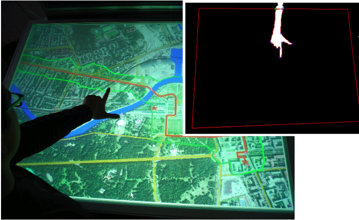
Fig. 10. Manipulation of the overview image with camera tracked hand gestures (small image)
