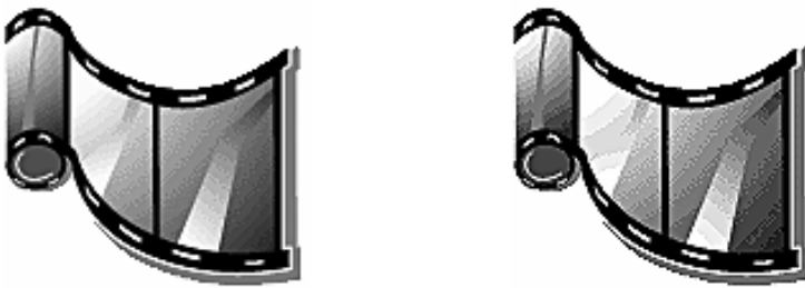
Fig. 7. An icon shown on an 8-bit display Fig. 8. An icon shown on a 4-bit display presenting 256 colors presenting only 16 colors
