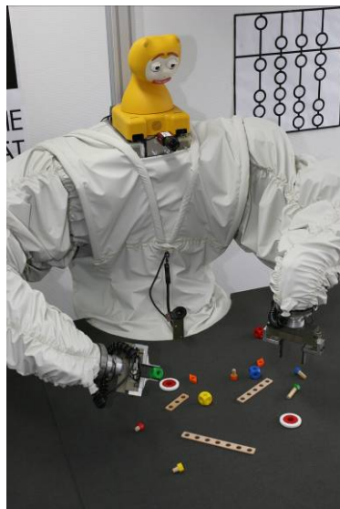
Fig. 2. Setup with two industrial robot manipulators and an animatronic head
