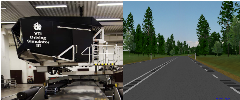
Fig. 1. Left: The moving base driving simulator at VTI. Right: A simulated road example.
