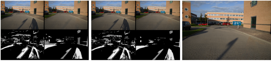
Fig. 3. Professional camera. RAW converted into bitmap. Manual settings. [Left] Low lambda ( \lambda = 1 ). [Middle] Higher lambda ( \lambda = 3 ). The photographers leg is segmented as full shadow, but the shadow from the small thin pole in front of the blue container is deleted by the over-smoothed non shadow region. [Right] The shadow of the photographer has been removed.
