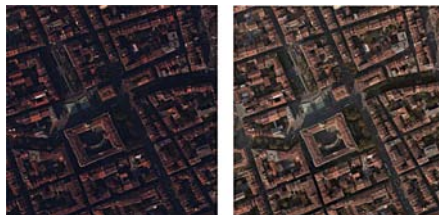
Fig. 2. RGB image representing downtown of Marseille before (left) and after (right) the atmospheric haze reduction
