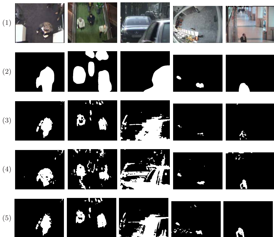
Fig. 6. Results obtained on 5 sequences with 4 algorithms: (1) Input sequence, (2) our algorithm, (3) smoothed temporal derivative, (4) non-parametric modeling, (5) difference-based spatiotemporal entropy
