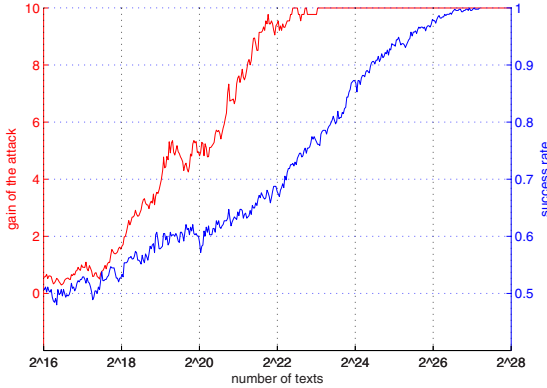
Fig. 7. Evolution of the gain and success rate w.r.t. the number of encrypted plaintexts
