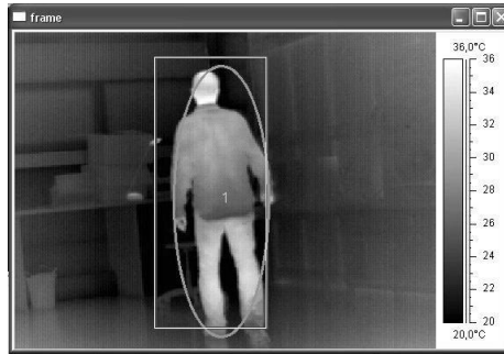
Fig. 7. A detection example, the rectangle is the human detection result in the blob neighborhood shown by the ellipse
