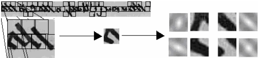
Fig. 3. Illustration of the sub windows extraction process and their corresponding autocorrelation functions
